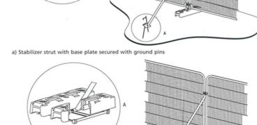
b) Stabilizer strut mounted on block tray
